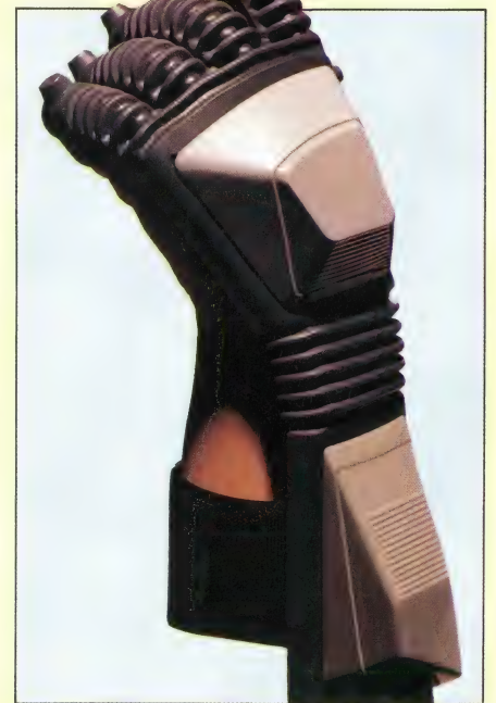
The 'Space Glove' enables interaction with objects in the virtual environment.
